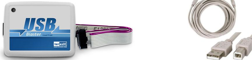
2. Connect one end of the USB-Blaster to a USB port on your computer. Connect the other end to the keyed 10-pin connector on the board whose FPGA or CPLD you wish to program. Power must be applied to the board. If the programmer has been installed already then skip to step 5.
