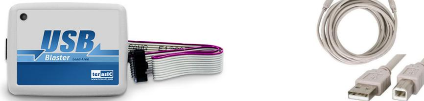
2. Connect one end of the USB-Blaster to a USB port on your computer. Connect the other end to the keyed 10-pin connector on the board whose FPGA or CPLD you wish to program. Power must be applied to the board. If the programmer has been installed already then skip to step 5.
